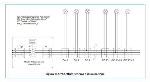
Figure 2 shows a public lighting system consisting of a three-phase switchboard and a single three-phase line. The changes to be made are described below.
